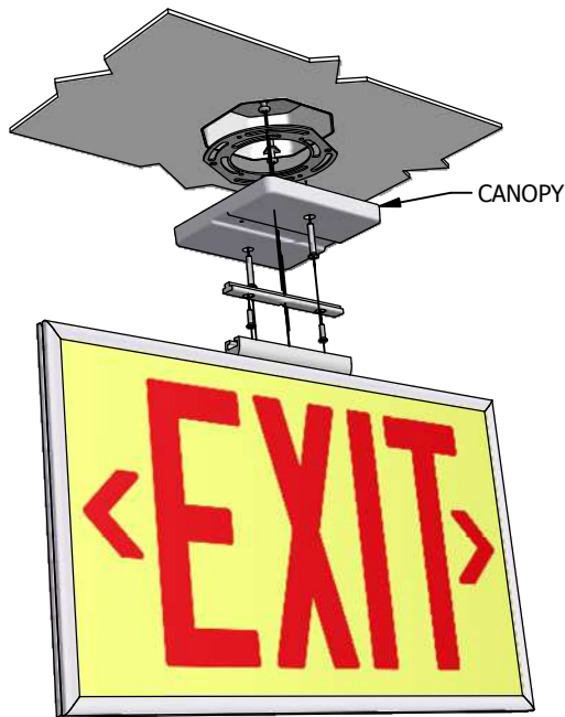
RETRO FIT INSTALLATION
